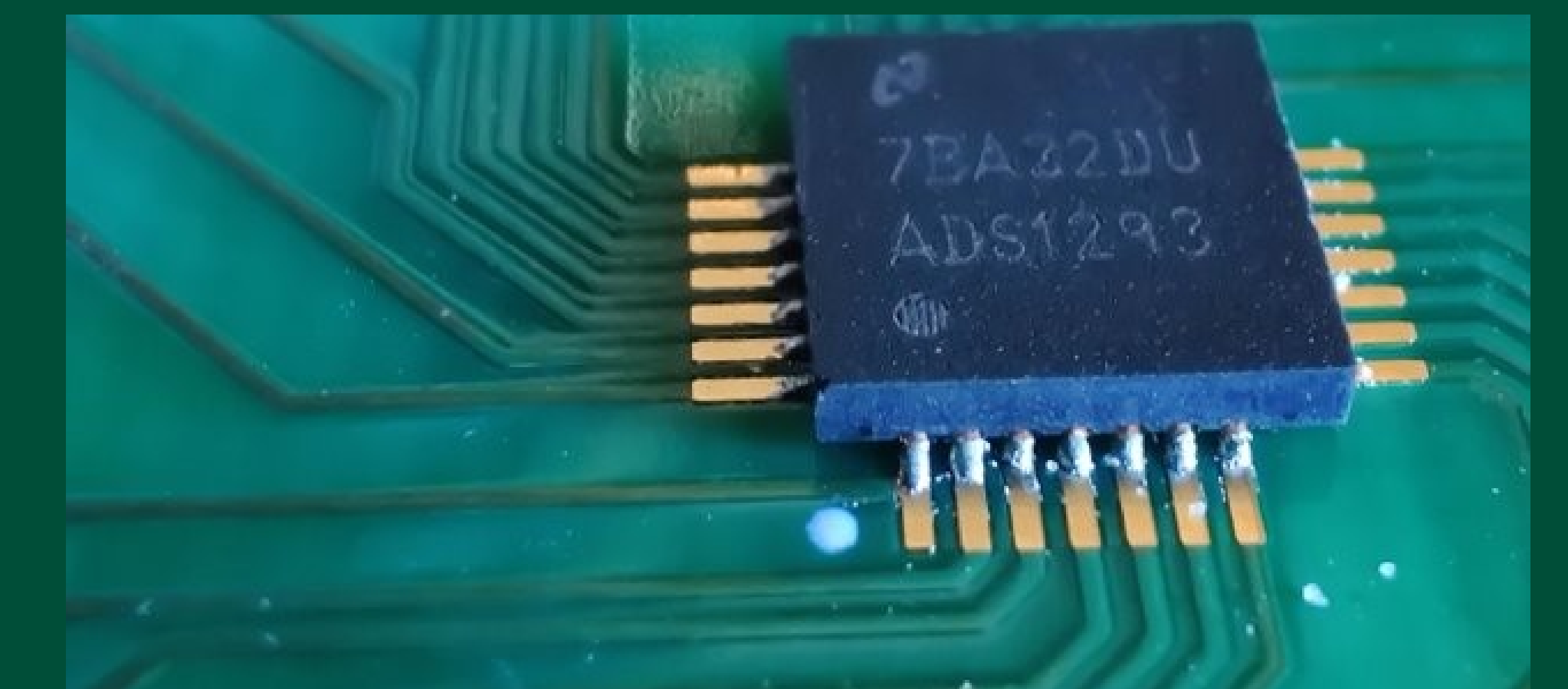
Figure 6: ADS1293 Electrocardiogram Instrumentation Device.
